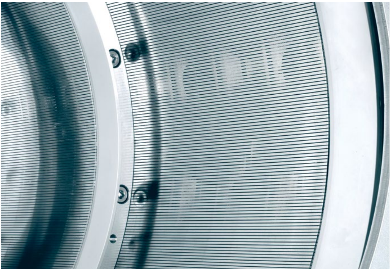
Wedge wire installed on a pusher centrifuge
