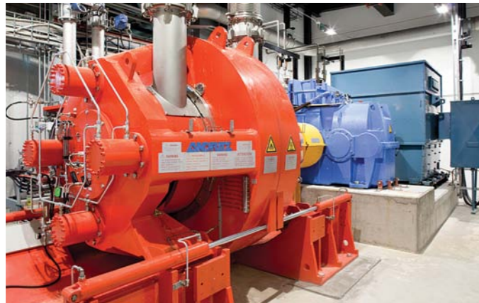
The world's largest LC refiner – the TwinFlo TF72 ▶
