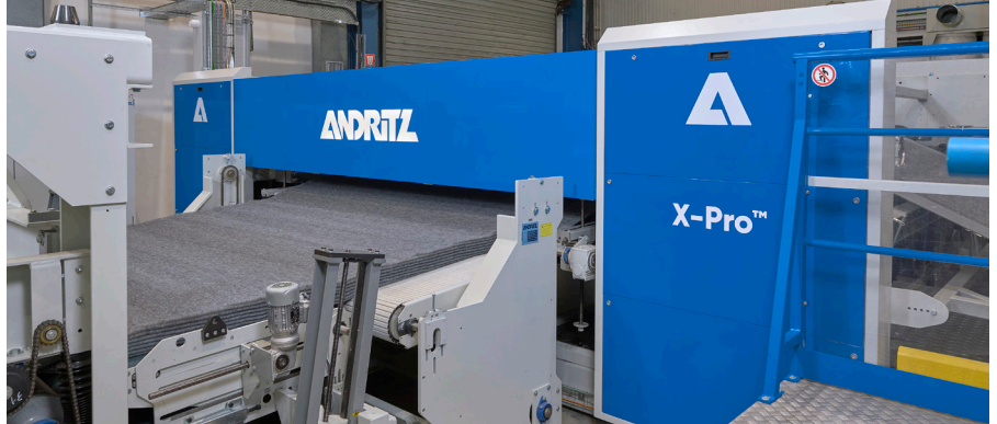
The new ANDRITZ X-Pro™ crosslapper installed on the ANDRITZ needlepunch pilot line
