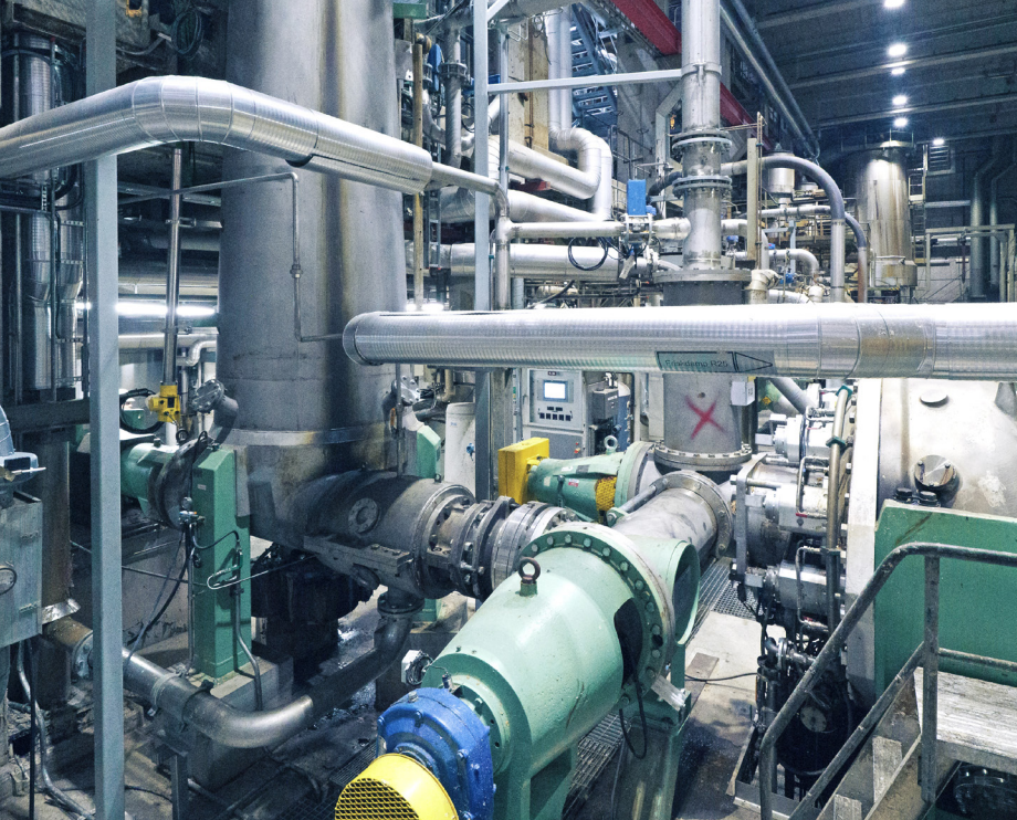
Skogn's TMP line with refurbished second-hand equipment.
