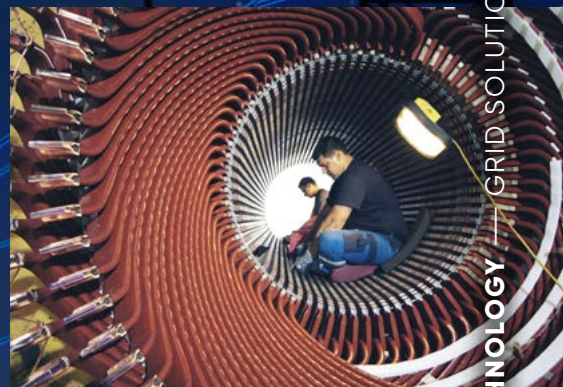
Manufacturing work on a turbo generator in the ANDRITZ workshop in Weiz, Austria
