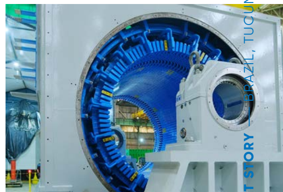
The synchronous condenser for Feijó during manufacturing.
