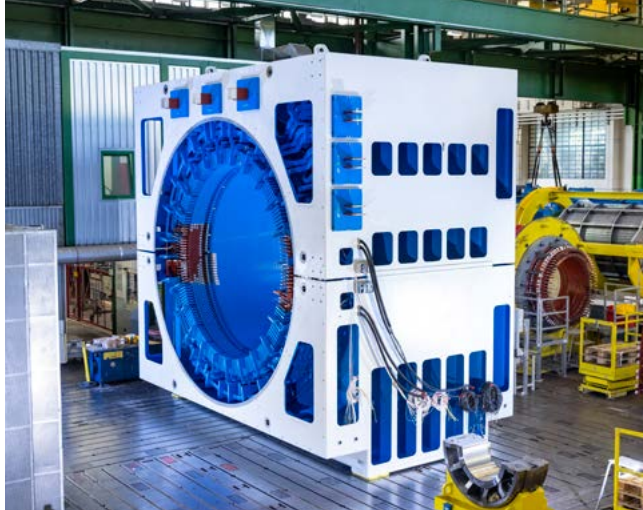
Synchronous Condenser manufactured for the EnergyConnect project in Australia. The component for Bakersfield will be nearly identical.
