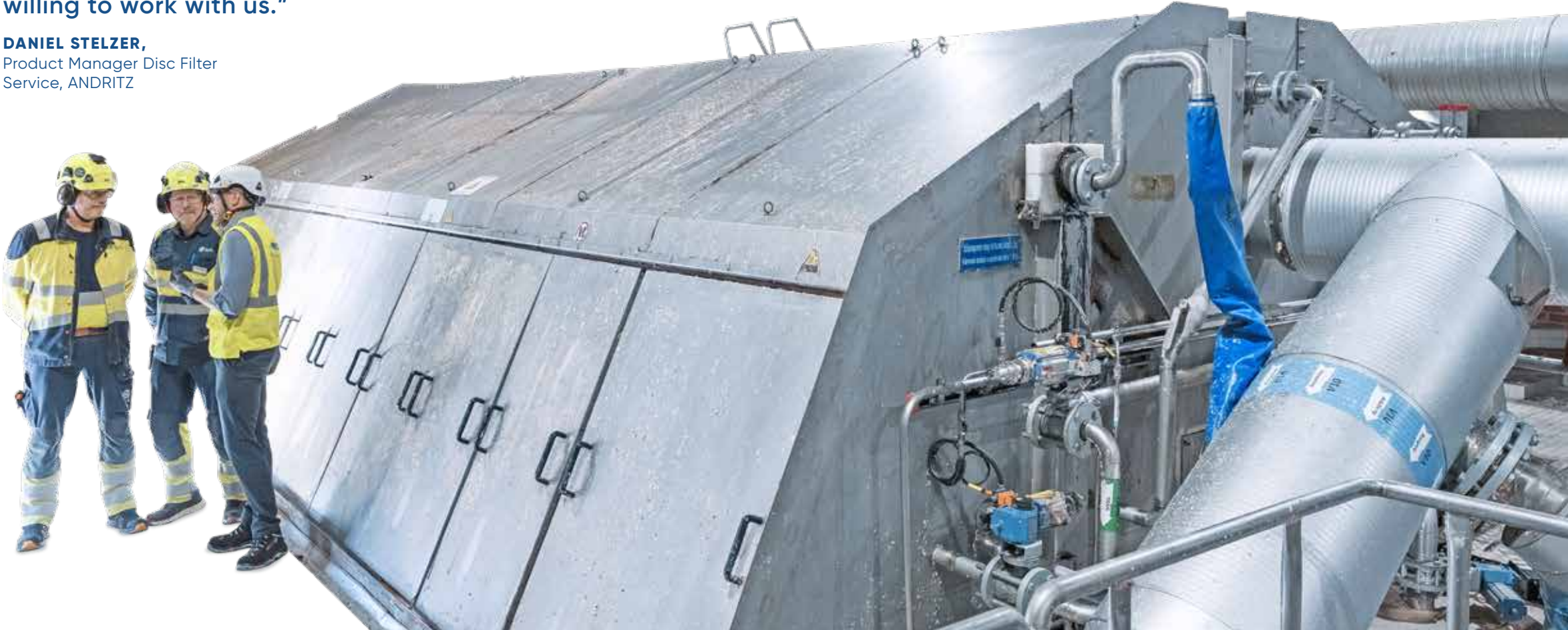
ANDRITZ upgraded SCA's disc filter in a way to handle a very wide range of fiber freeness profiles.
