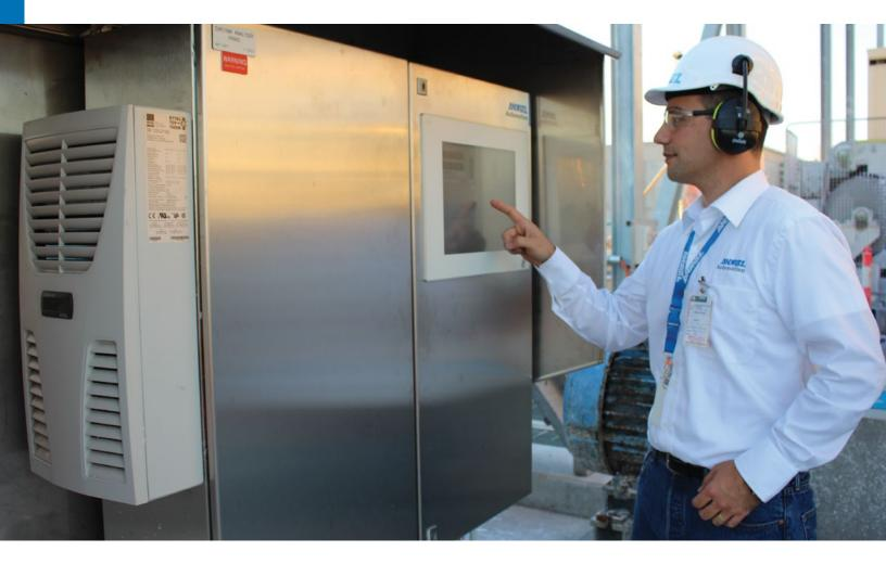
ANDRITZ PulpVision is a continuous pulp analyzer for the pulp and paper industry. The analyzer is equipped with a high-speed camera for pulp image capture and machine learning software for data analysis. PulpVision is installed in a bypass loop of the online process to quantify contaminants such as: stickies, dirt, Styrofoam, etc. The measurement principle is based on a composite of multiple attributes, including color, reflectance, and translucence.
