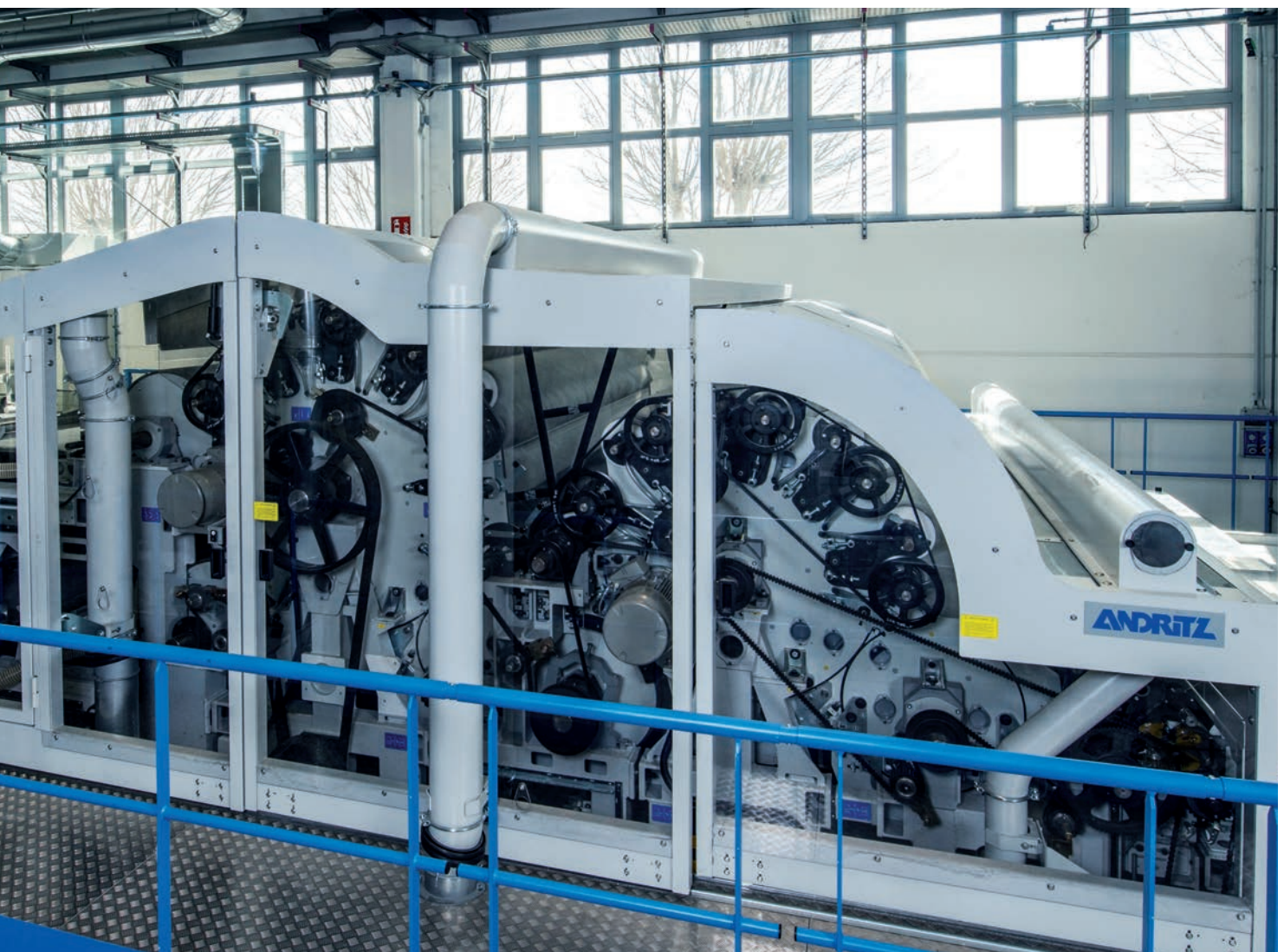
ANDRITZ carding machine in operation
