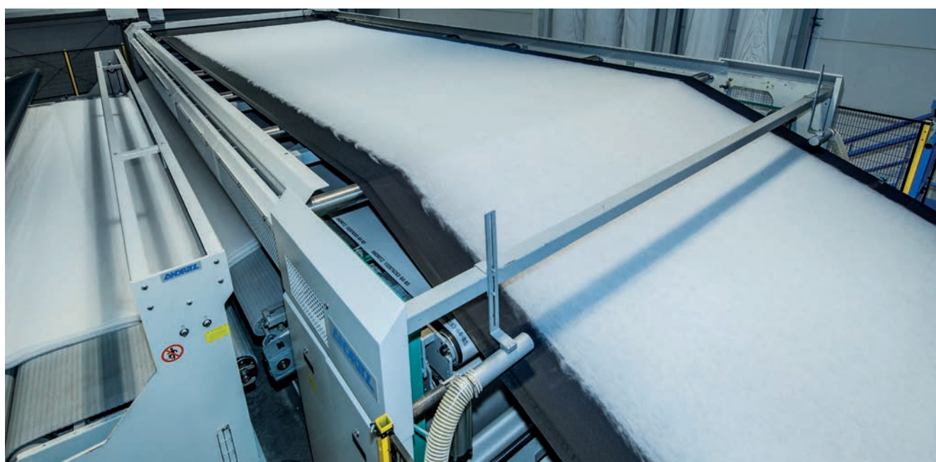
ANDRITZ crosslapper in operation
