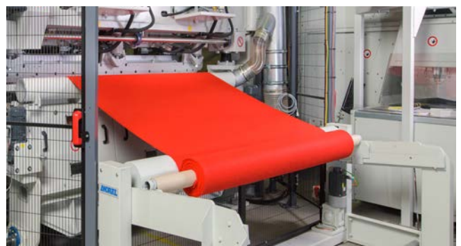
ANDRITZ neXloom needleloom velour SDV 2+2 exit view
