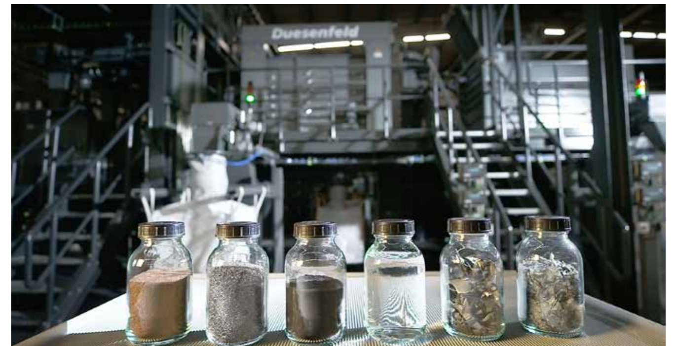
Main output fractions (left to right): Copper foil, aluminium foil, black mass, solvents, heavy parts, separator foil © Duesenfeld
