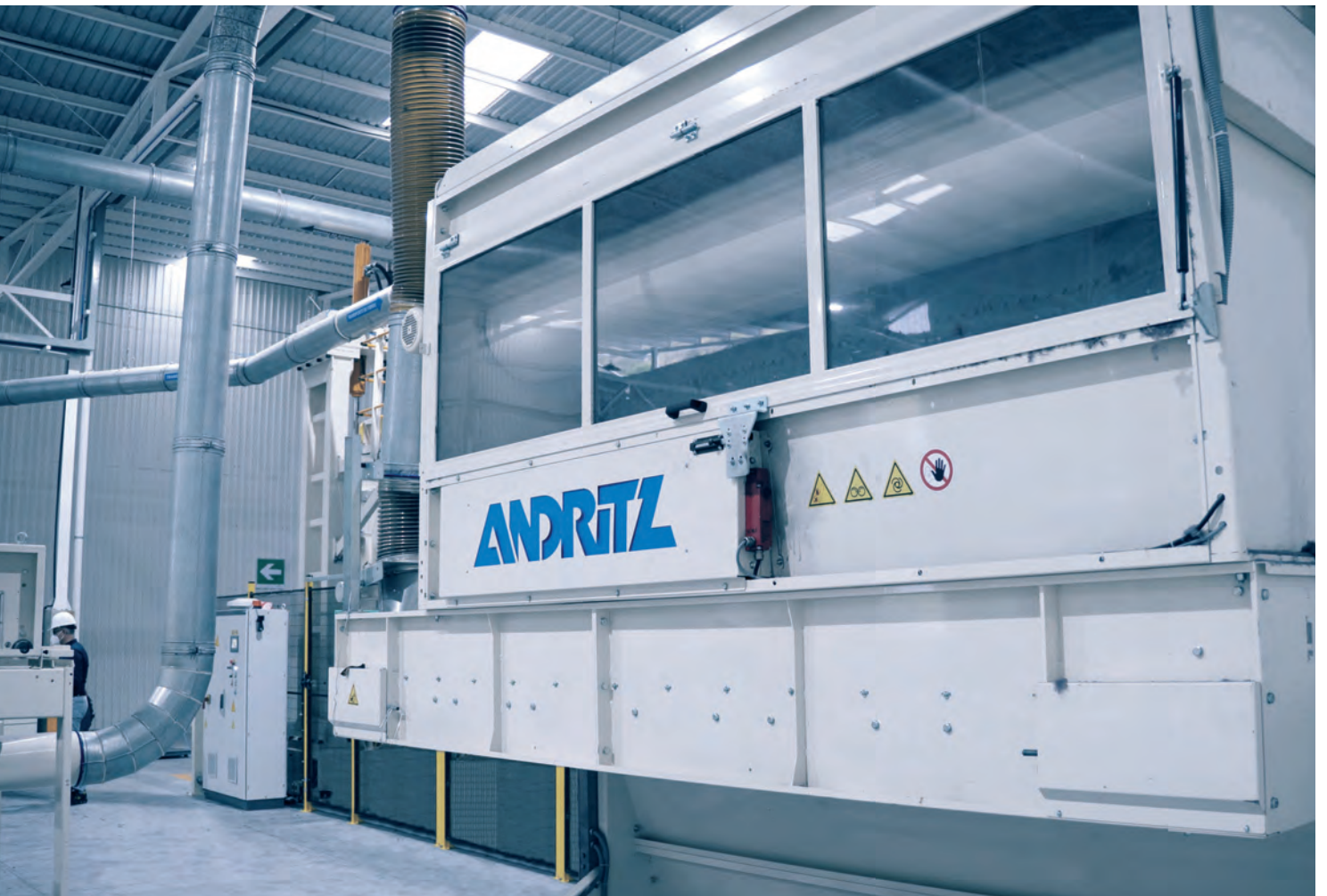
Blending box for optimal fiber blend homogeneity
