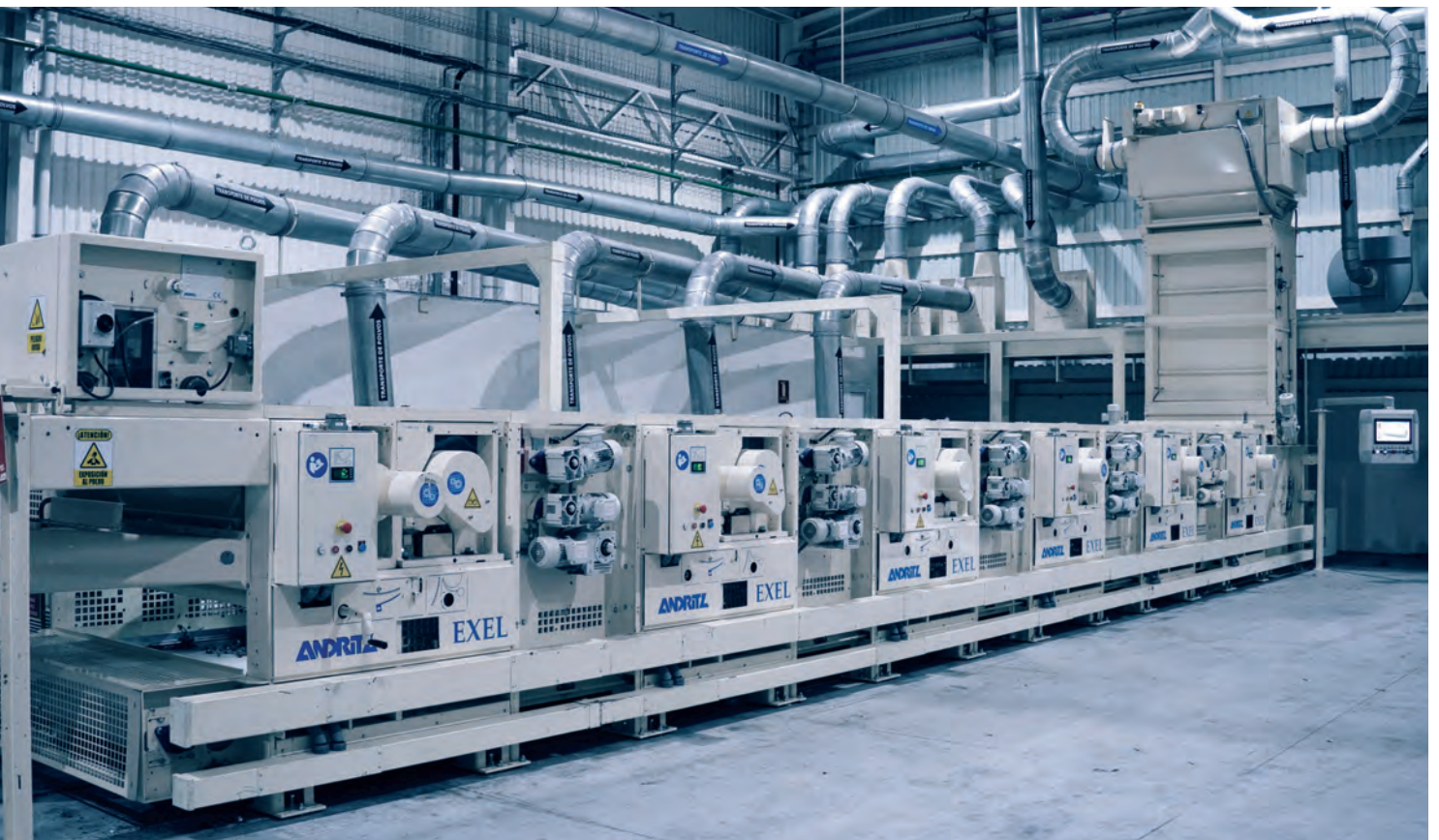
Exel tearing machine for medium-range capacities
