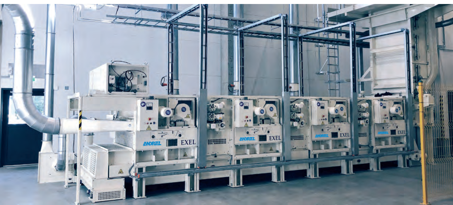
Exel tearing machines in operation
