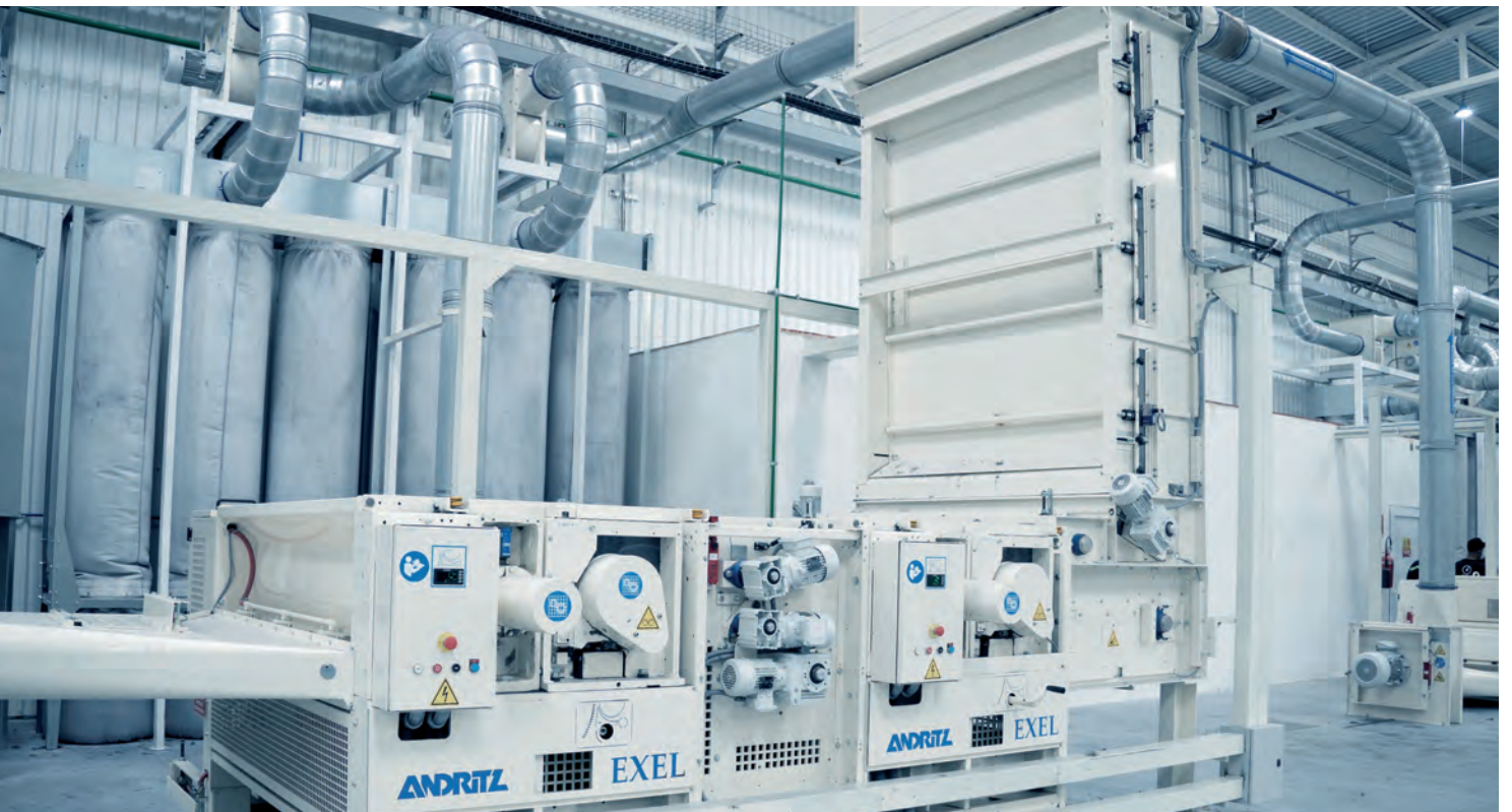
Picker shredder for pre-opening and cleaning
