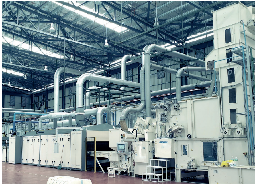
Airlay line with an oven in operation
