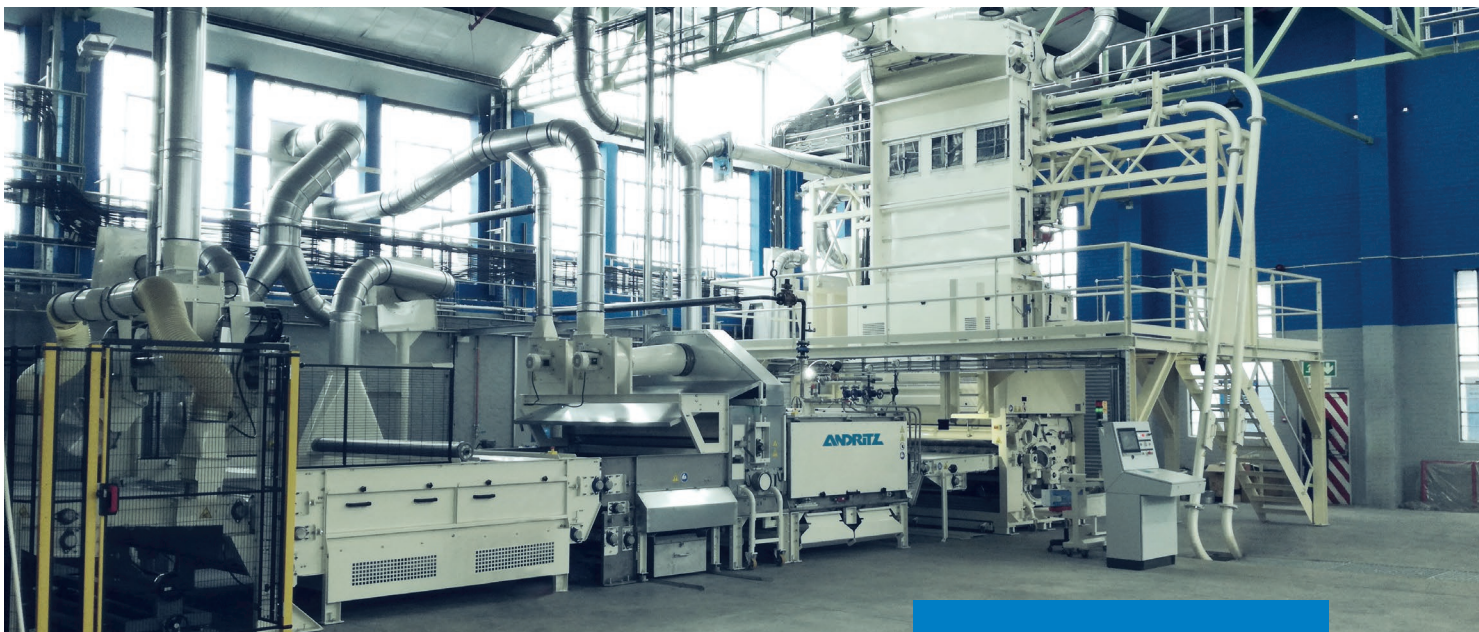
Airly resinfelt line in operation
