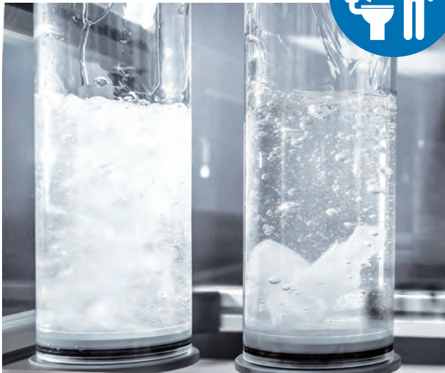
Flushability test at ANDRITZ technical center in Krefeld, Germany
