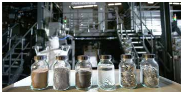
Output materials from the battery recycling process (left to right): Cooper foil, aluminium foil, black mass, solvents, heavy parts, separator foil © Duesenfeld
