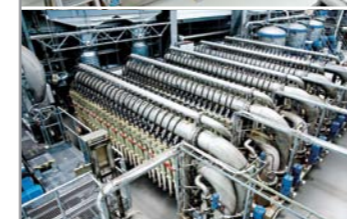
AhiCleaner high-density, light-weight and throughflow cleaners
