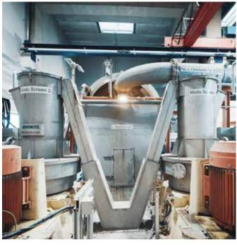
The ModuScreen TD is available in two sizes, featuring installed power up to 110 kW.
