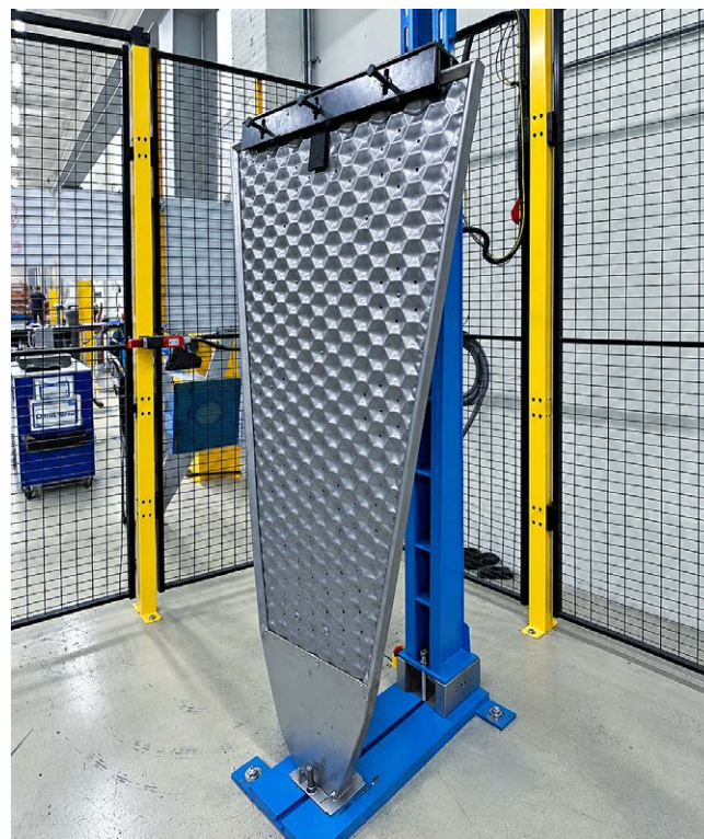
Lifetime validation with bending and deflection test
