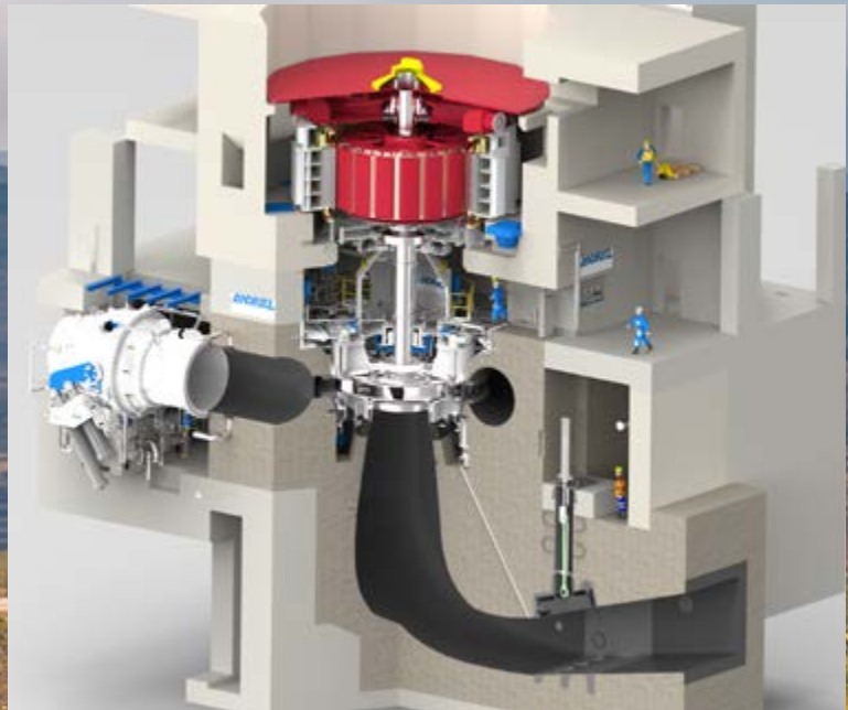
3D rendering of a pump turbine unit including motor generator, pump turbine, and inlet valve.
