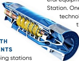
technological advantages of the suggested ANDRITZ solution to meet the special technical requirements is the use of submersible motor pumps in double-suction design. For this purpose, two impellers rotating in opposite directions are arranged one above the other and driven continuously by a pump shaft. This compensates in full for the axial thrust, regardless of the rotation speed. The hydraulic thrust forces acting on the pump, the motor, and the axial bearings, are completely neutralized.
