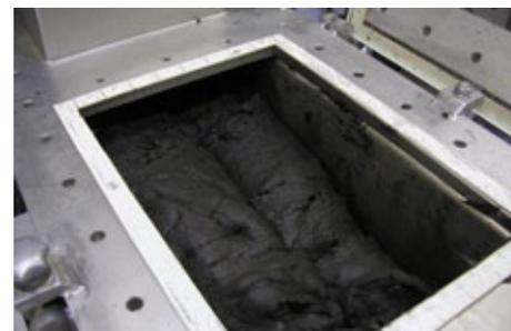
The ANDRITZ Gouda paddle dryer also has many references for full drying (90% dry solids) based on a once-through drying process without back-mixing. The plastic phase in sludge around 45-60% DS never causes problems in this dual shaft machine. The self-cleaning effect of the two shafts with intermeshing paddles deals easily with the plastic phase without any difficulty.
