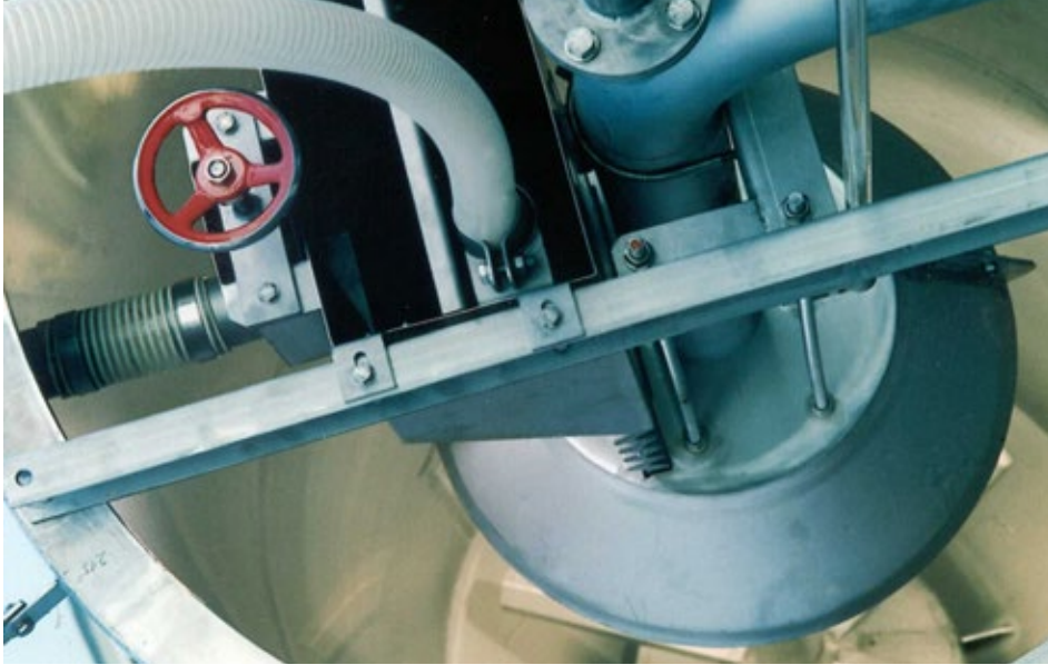
▲ Inside sand wash box of stainless steel version
