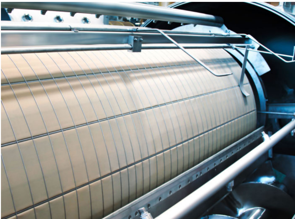
▲ Krauss-Maffei TDF pressure drum filter with open housing
