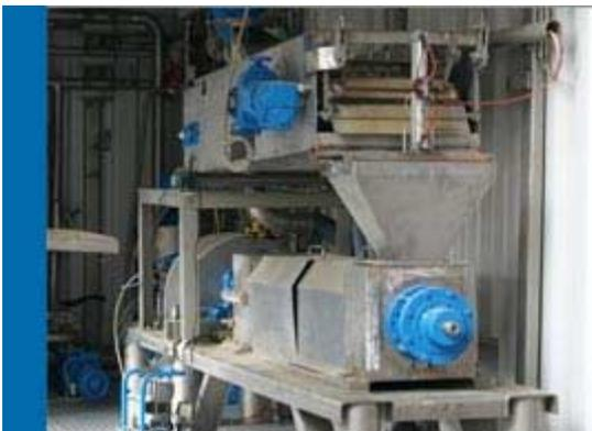
**Gravity table and sludge screw press
