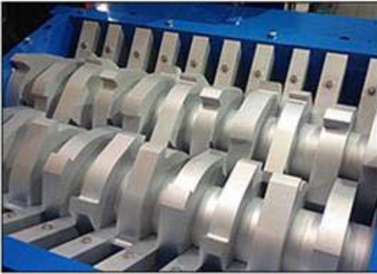
Cutting unit of the ANDRITZ Rotary Shear UC
